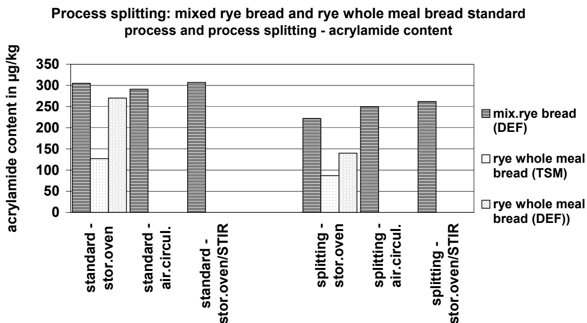
Figure 7: Reduction of the acrylamide content of mixed rye bread and whole meal bread by baking splitting in different baking ovens (STIR = storey oven with selective infrared radiation; air.circul. = air circulation /shop oven or rack oven; TSM = dough acidifier; DEF = Detmold one-stage method)
